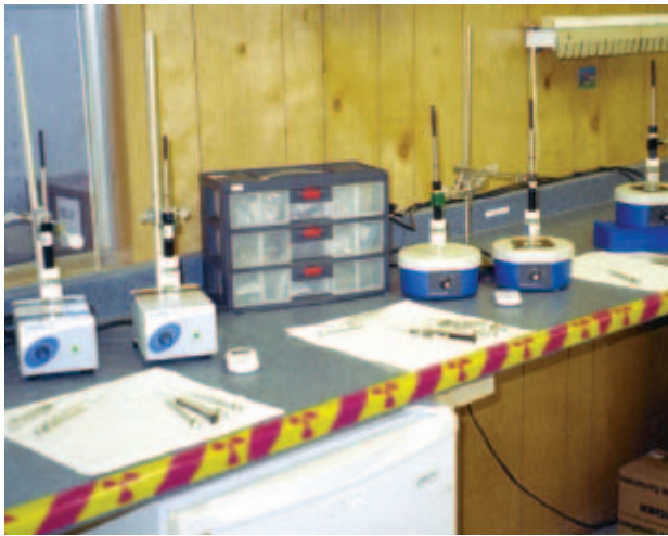
SPME equipment is extremely user friendly and requires very little space. As shown in this photo, a single bench top (2'x 6') accommodates 5 simultaneous sample extractions.
