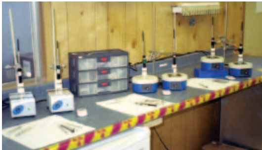
Extraction: 6 minutes using SPME
