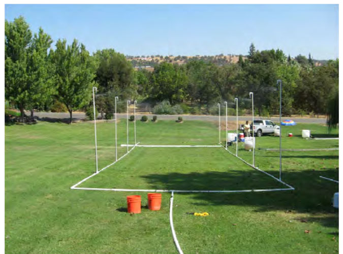
A rainfall simulator was set up to represent a winter rainstorm.
