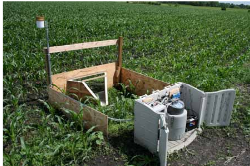
A runoff monitoring station at a paired watershed study in Minnesota. The two-foot H-flume is discharging through a "side inlet". See the full story on page 3.
