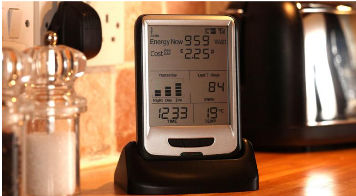
Figure 3. A consumer-grade electricity monitoring device that can track and store data from up to ten different energy using devices. Photo courtesy Current Cost Ltd.
