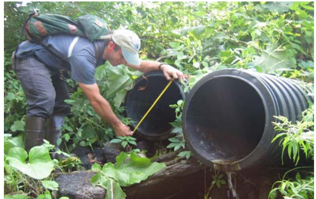
A scientist measures an outfall pipe found while searching for sources of illicit discharges into Vermont waterways.
