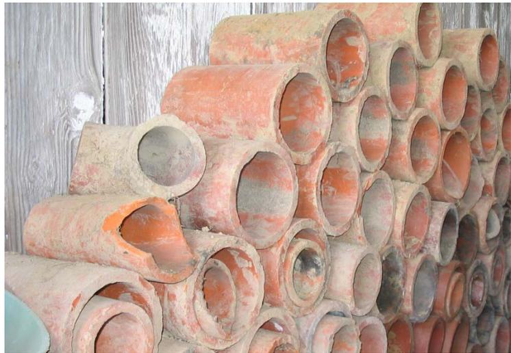
Figure 1. Old drainage tile sections on an Ohio farm.
