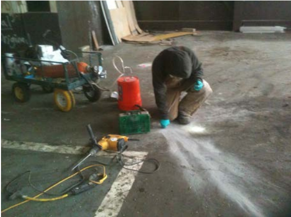
Stone field staff performing dynamic soil gas investigation.
