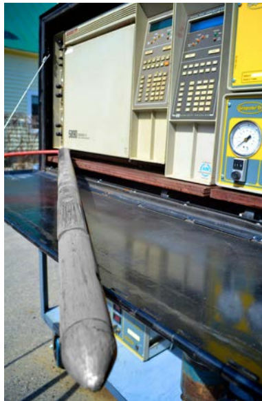
The Membrane Interface Probe (MIP) provides real-time data to assess source zones and plume cores.
