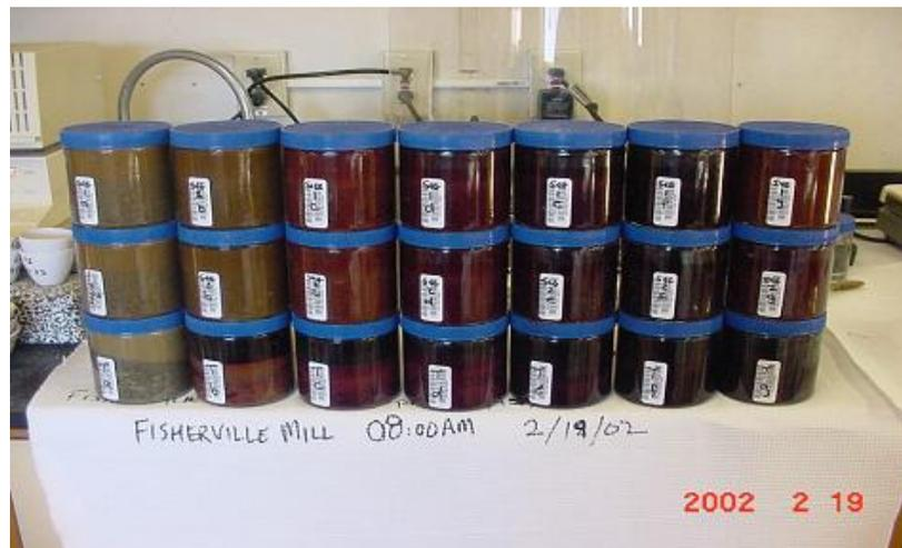
*Figure 21. Sodium Permanganate Bench-Scale Treatability Testing*
