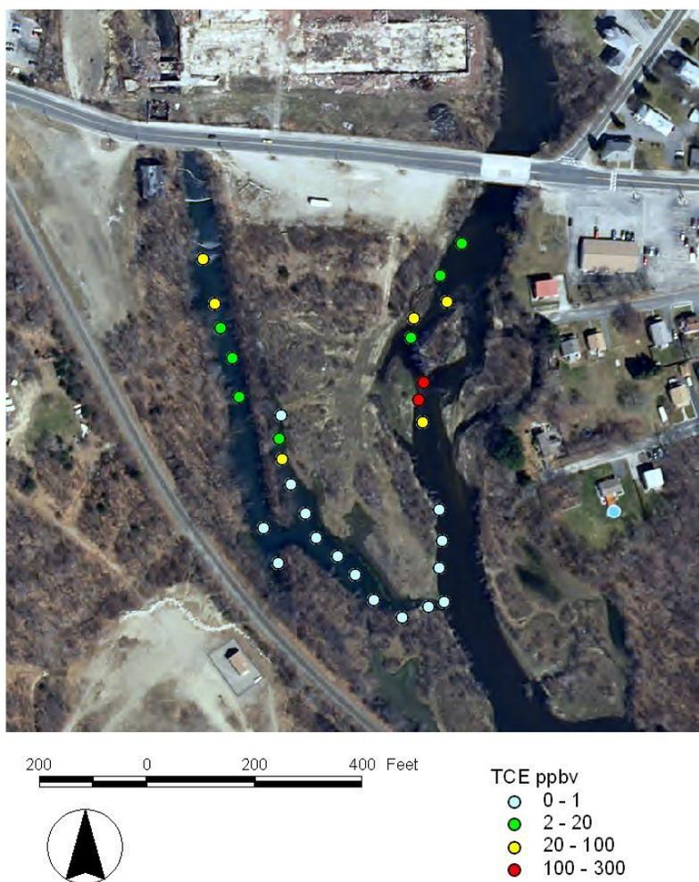
*Figure 8.* TCE concentrations measured in passive vapor diffusion samplers (ppbv) in June 2000.
